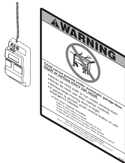
FIG. 3-5 Mounting Entrapment warning label
