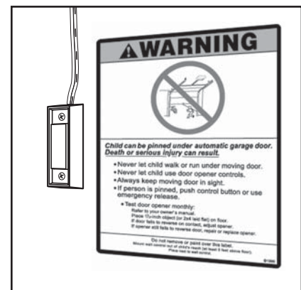
FIG. 3-5 Mounting Entrapment warning label.
